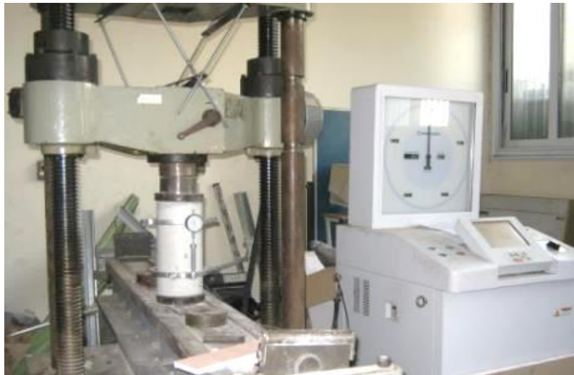
Figure 8: Test set-up for elastic modulus test
