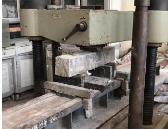
Figure 7: Test set-up for flexural strength test.
