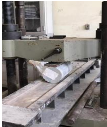
Figure 6: Test set-up for splitting tensile test.
