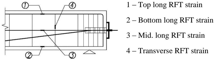
**Figure4** : Arrangement of the steel strain gauges for the specimens
