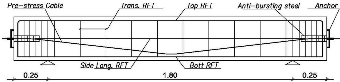
**Figure 1:** Details of reinforcement for four specimens
