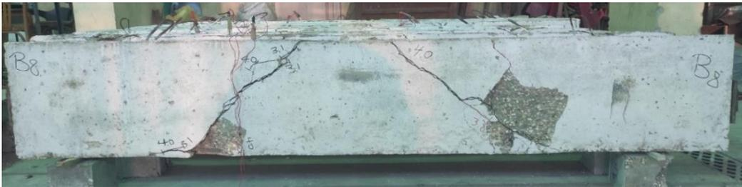
**Figure 6:** Crack patterns at failure of specimen (B8)
