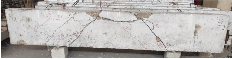
**Figure 8:** Crack patterns at the failure of specimen (B9)
