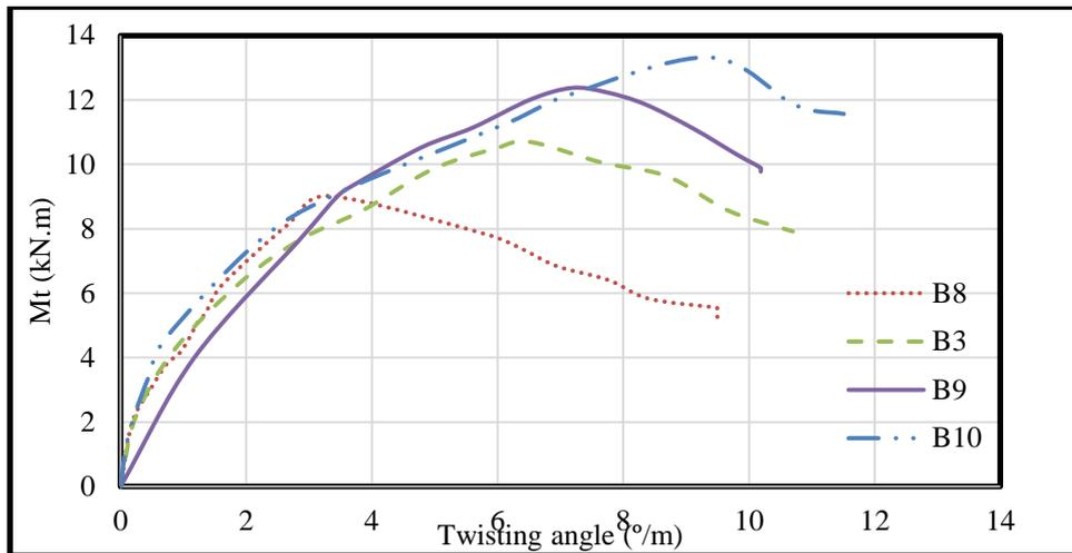
**Figure 11:** Torsional Moments - twisting angle curve.
