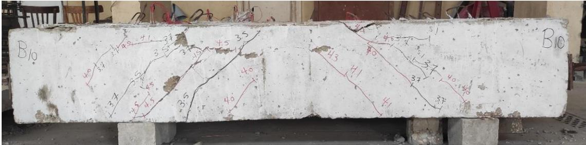
**Figure 9:** Crack patterns at failure of specimen (B10)
