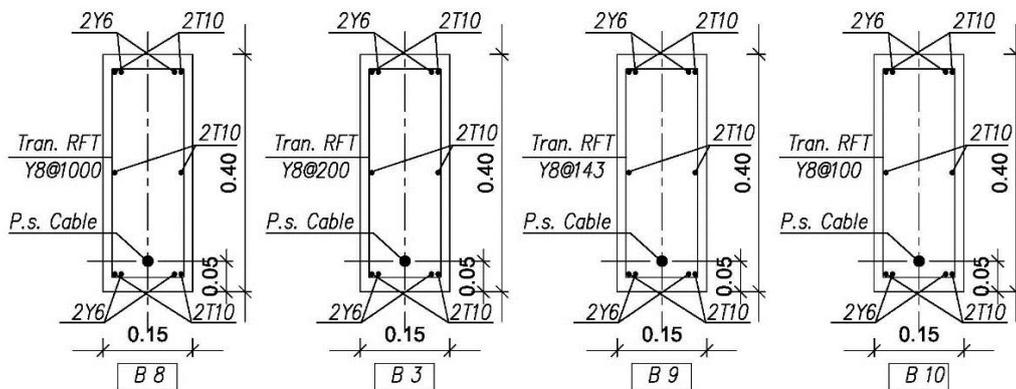
**Figure 3:** Details of reinforcement for all specimens.
