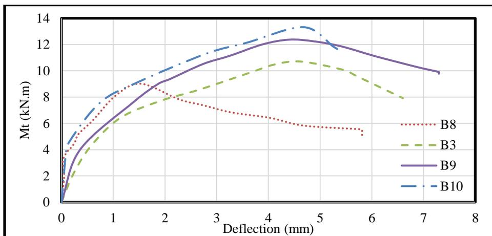
**Figure 10:** - Torsional Moments – deflection curve of tested specimens.
