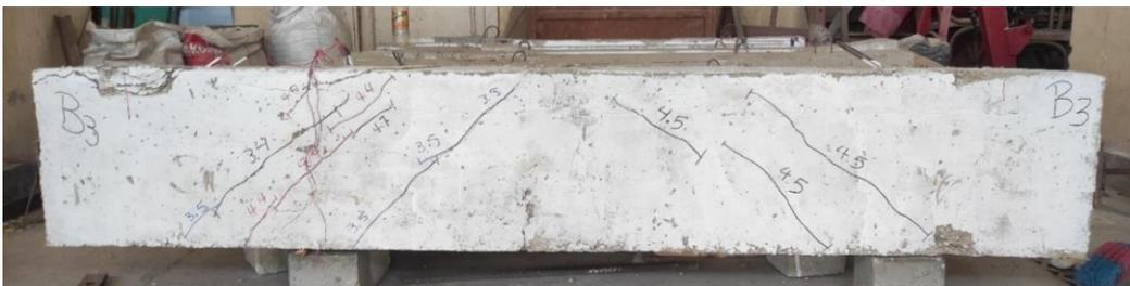
**Figure 7:** Crack patterns at failure of specimen (B3)
