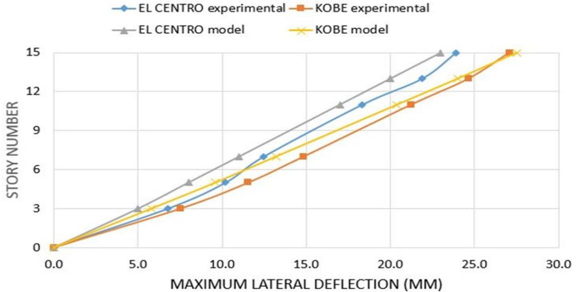
**Figure 3:** shows a good resemblance between the results obtained from the analytical model and the experiment
