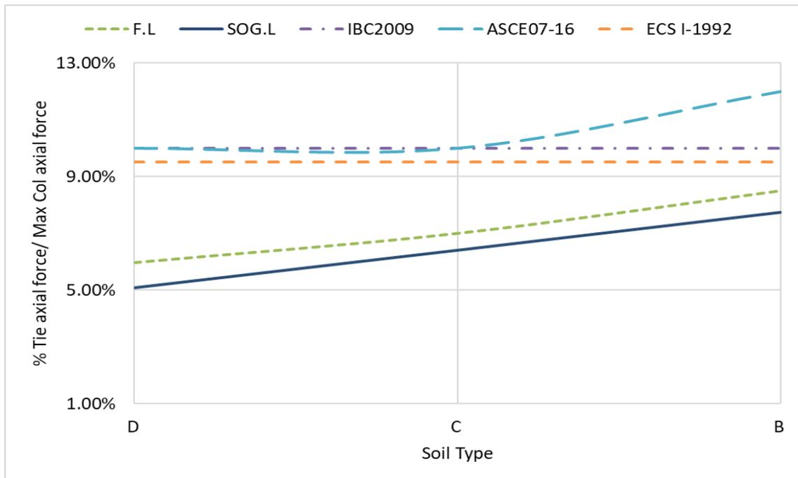
**Figure 10:** The relationship between the percent Tie axial force / maximum column axial force and Soil Type
