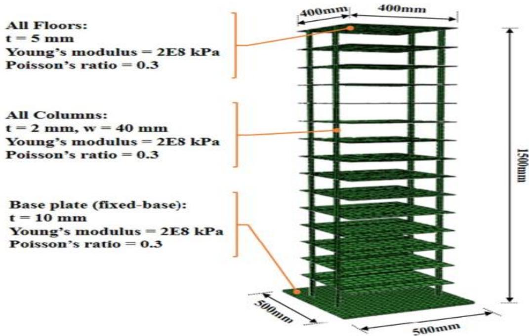
**Figure 1:** 3D numerical model of this scaled frame structure in ABAQUS presented in (Xiaofeng Zhang and Harry Far 2021). [6]
