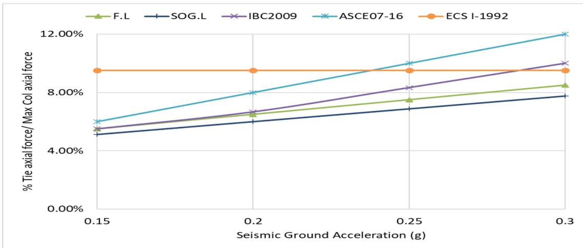
**Figure 11:** The relationship between the percent Tie axial force / maximum column axial force and maximum seismic ground acceleration
