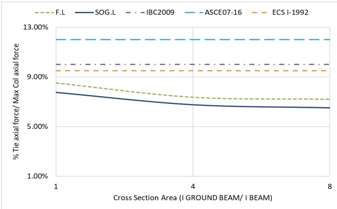
**Figure 14:** The relationship between the percent Tie axial force / maximum column axial force and tie beams cross section area
