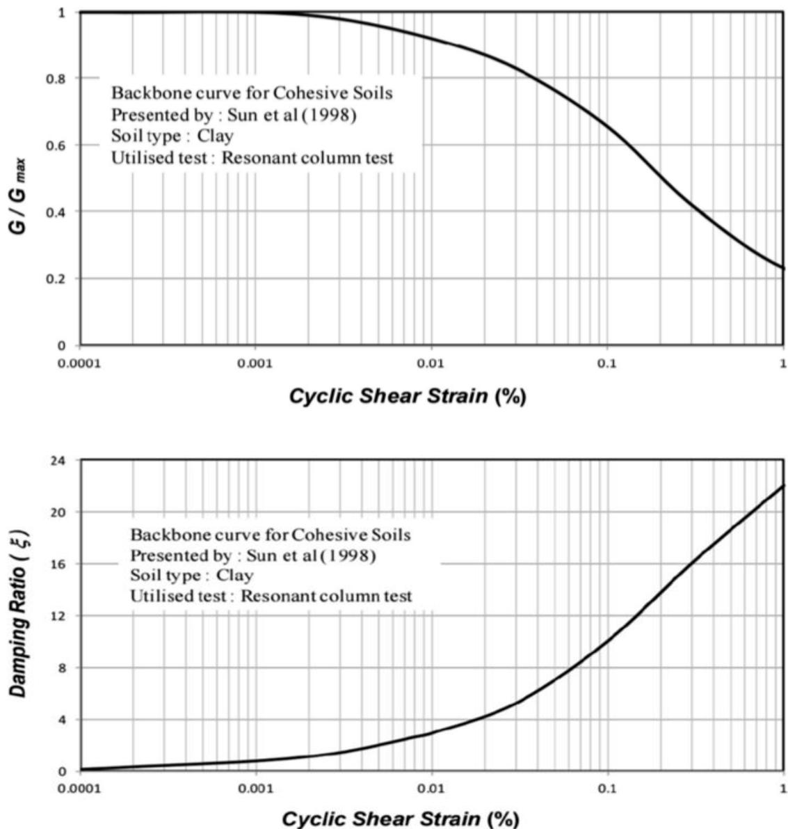
**Figure 5:** The first graph depicts the Relationship between  $G/G_{max}$  versus  $\gamma_c$  for cohesive soils, while the second graph depicts the Relationship between  $\xi$  versus  $\gamma_c$  for cohesive soils (Presented in (Joseph Sun., H. B. Seed 1998)) [13].
