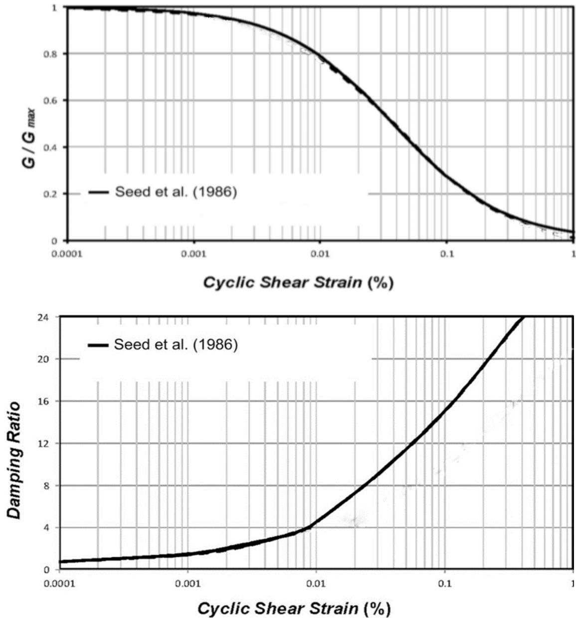
**Figure 6:** The first graph depicts the Relationship between  $G/G_{max}$  versus  $\gamma_c$  for cohesionless soils, while the second graph depicts the Relationship between  $\xi$  versus  $\gamma_c$  for cohesionless soils (presented in (H. Bolton Seed, F. ASCE 1986) [12]).
