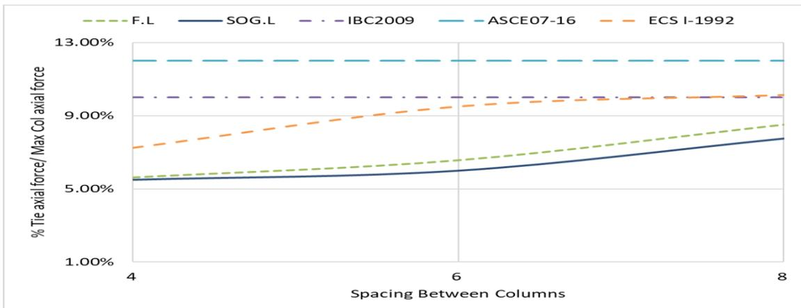
**Figure 12:** The relationship between the percent Tie axial force / maximum column axial force and the spacing between columns
