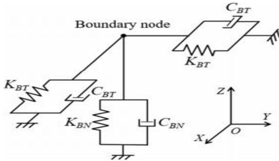
Figure 2: Viscous-spring boundary presented in (Liu Jingbo and Du Yixin 2006) [5].
