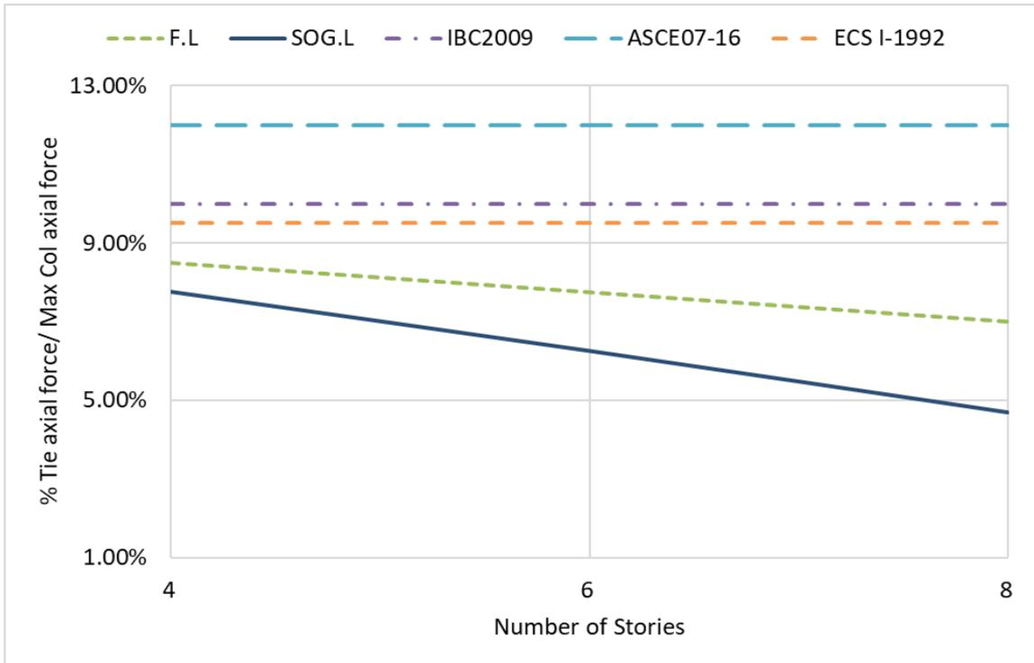
**Figure 13:** The relationship between the percent Tie axial force / maximum column axial force and the number of stories
