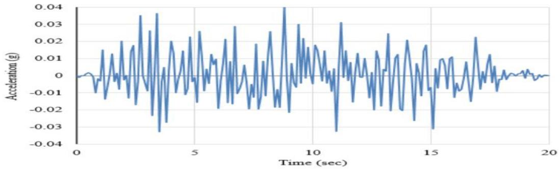
**Figure 4** Time-acceleration history of the artificial earthquake
