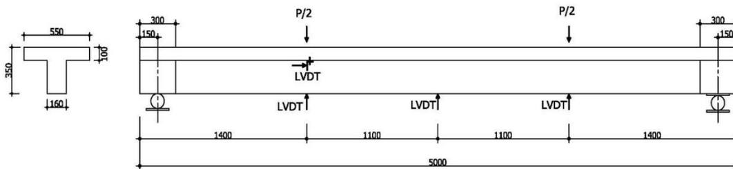
Figure (1): Details of Location of Applied Load and LVDT for (G1 – G2)
