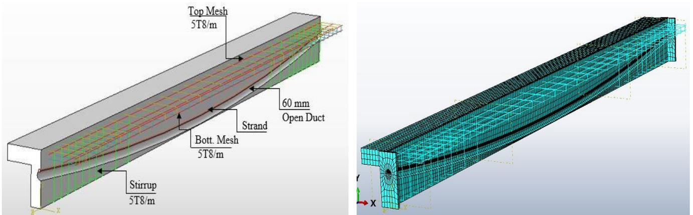
Figure (5): Typical Half Beam Detailed, Meshed with Simulated the Strand Curvature, End Anchor and Reinforcement.
