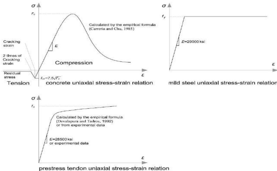
Figure (3): Finite Element Modeling Uniaxial Stress-Strain Models
