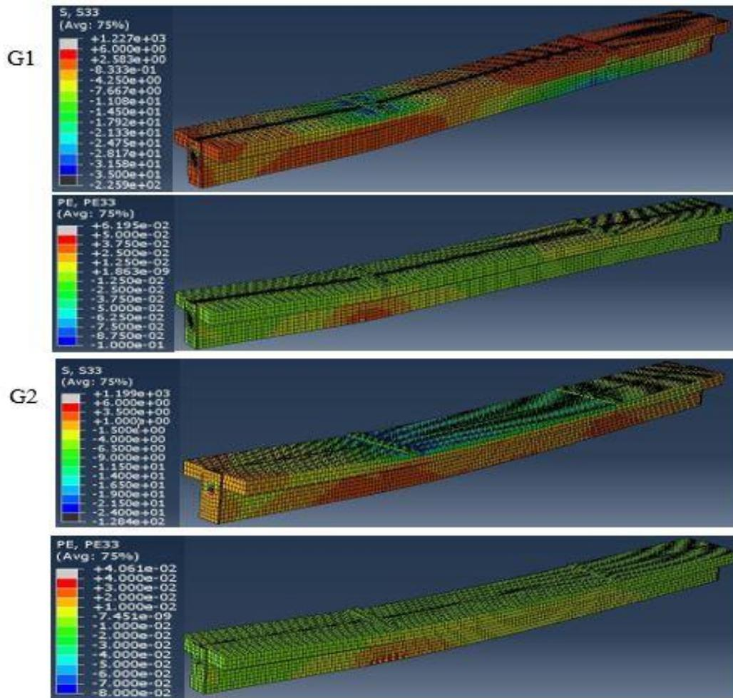
Figure (8): FE modelling Results of Concrete Stress and Strain at the Failure Loading G1 and G2
