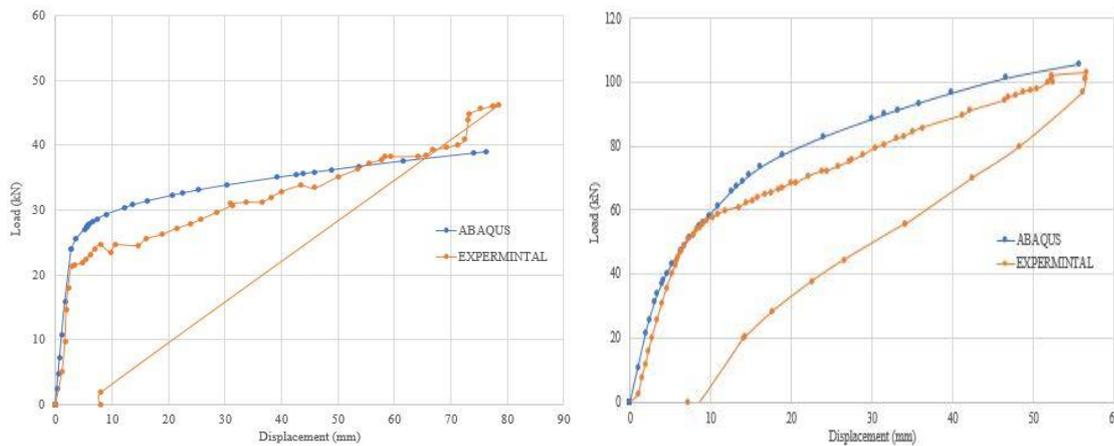
Figure (6): Comparison of Numerical and Experimental Load-Deflection Curve Specimen's G1 and G2
