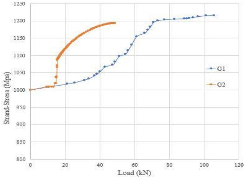
Figure (7): Comparison of FE modelling results of tendon Stress Increases Vs. Applied Load for G1 and G2
