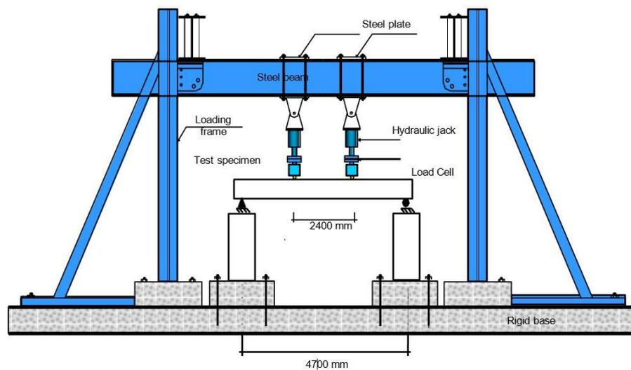
Figure (2): Test Setup for Tested Beams
