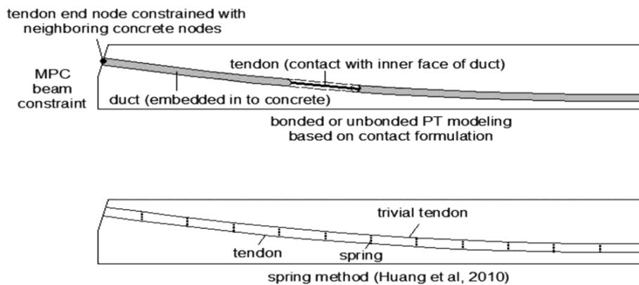
Figure (4): Modeling Details for Bonded or Unbonded PT tendons.
