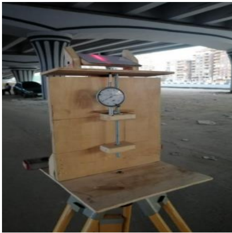
Figure (1) Reflectorless target with slope 1:2
