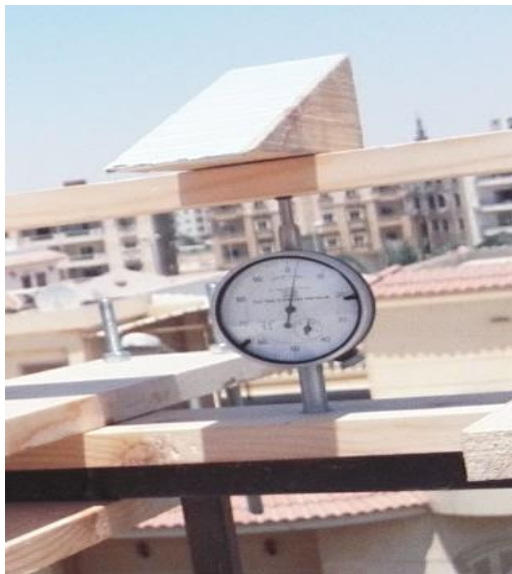
Figure (3) dial gauge below Reflectorless target
