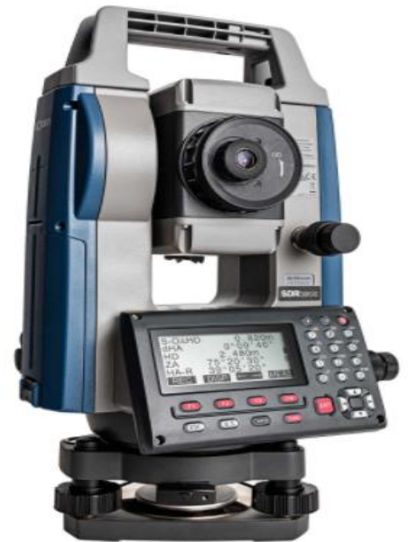
Figure (4) Sokkia with precise 7'' second
