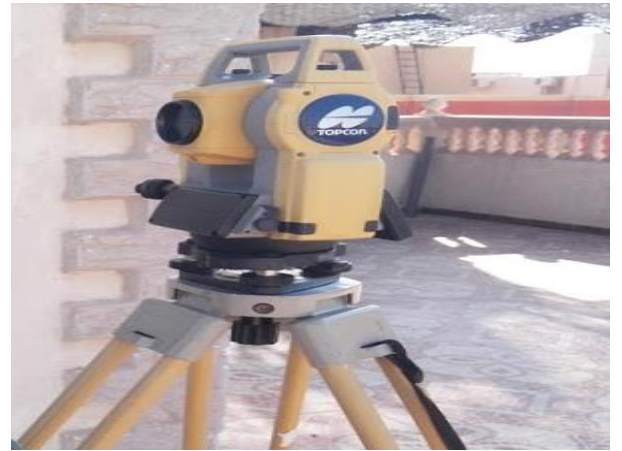
Figure (2) Topcon GTS with precise 7'' second
