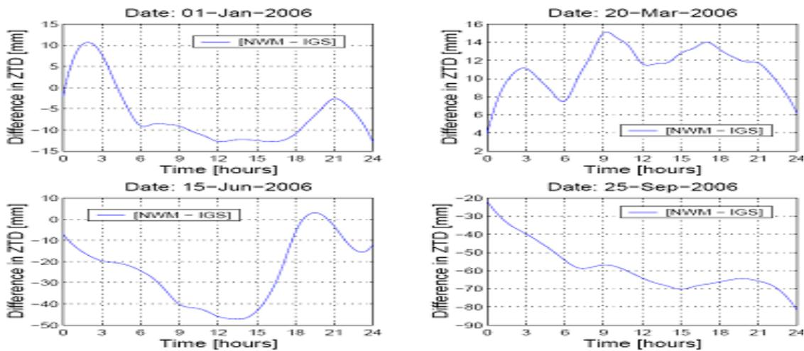
Fig. 1. The difference in zenith tropospheric delay between the suggested model's output and the IGS products at the METS, Finland, IGS station.
