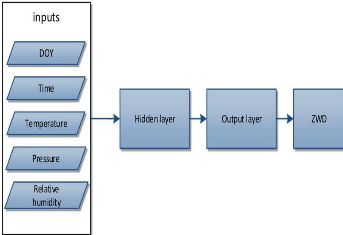
Fig. 3. Artificial neural network model design.
