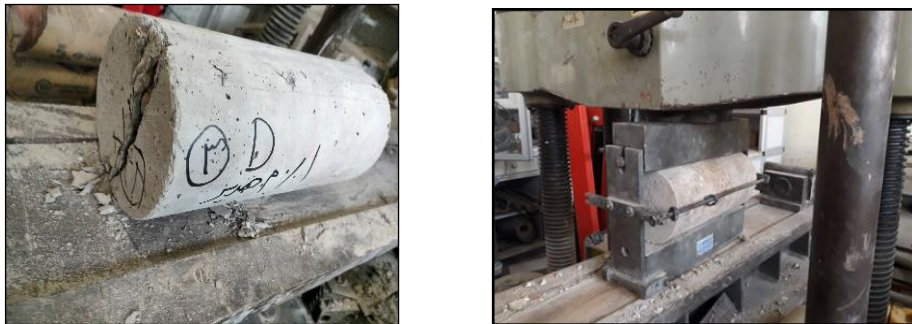
Figure (5): Splitting Tensile Test
