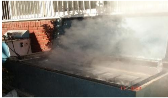
figure (4): Steam curing tank
