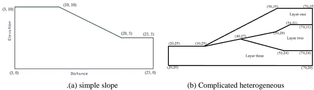
Figure 3 simple slope and Complicated heterogeneous slope geometries
