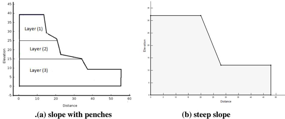
Figure 4 slope with penches and steep slope geometries
