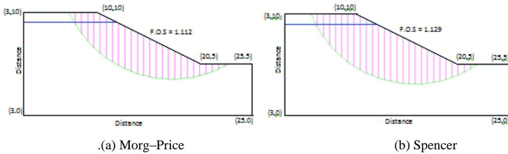
Figure 6.a, b soil in 2D with 1.0 m water depth below the surface with Morgenstern–Price and Spencer
