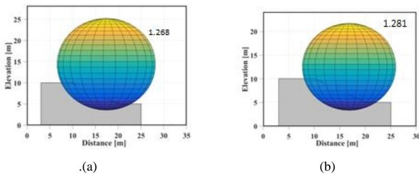
Figure 8.a, b 3D dry soil with Morgenstern–Price and Spencer critical slip surface
