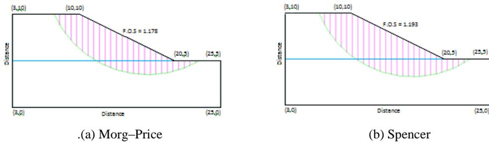
Figure 7.a, b water depth in the middle of the surface with Morgenstern–Price and Spencer
