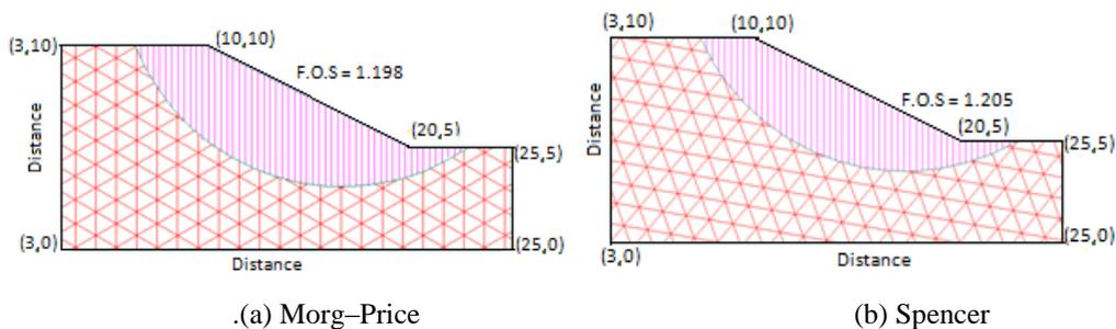
Figure 5.a, b dry soil in 2D slip surface with Morgenstern–Price and Spencer
