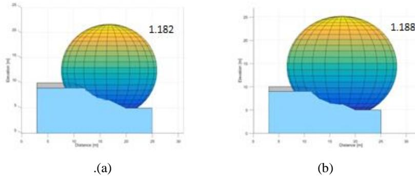
Figure 9.a,b 3D with 1.0 m water depth below the surface by using Morgenstern–Price and Spencer
