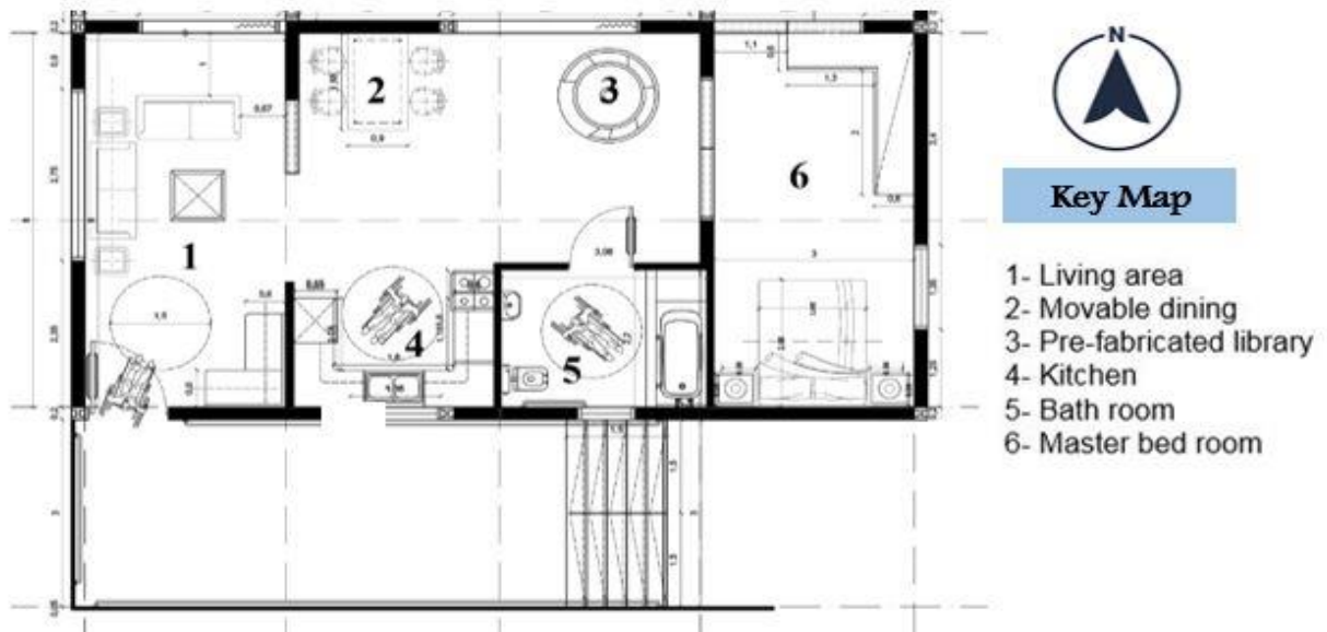
Figure 8: Ground floor plan (N.T.S) before extension with an area of 108 m 2 . (By researcher)
