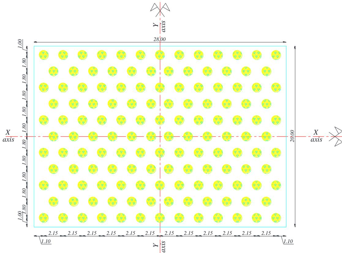
Figure 5: Stone column arrangement
