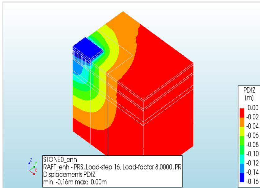
**Figure 8: Contours of vertical settlement under uniform load of 80 kPa**
