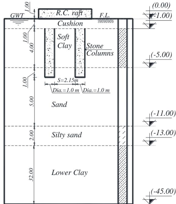
Figure 4: Soil stratification
