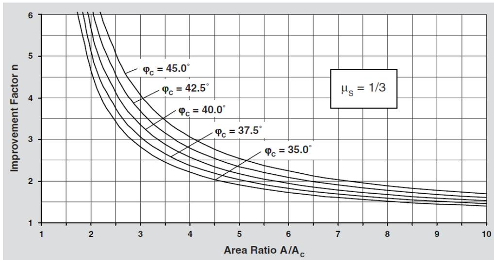
Figure 1: Design chart for vibro replacement (Priebe, 1995)
