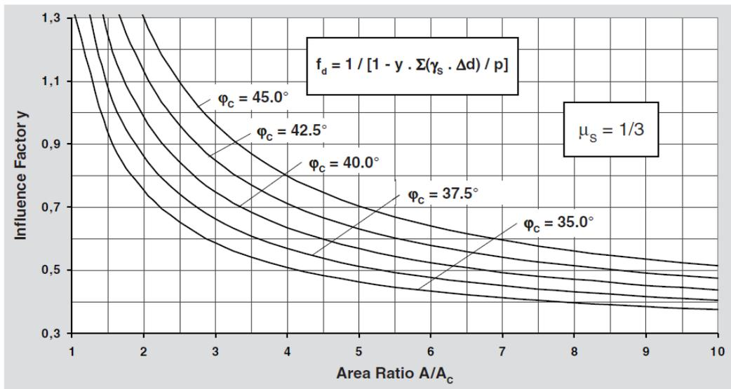
Figure 3: Determination of the depth factor (Priebe, 1995)
