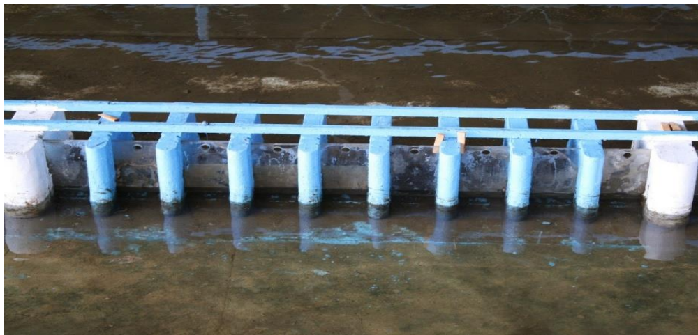
Photo 2: The Trash Rack Simulates 100% Blockage By Aquatic Weeds
