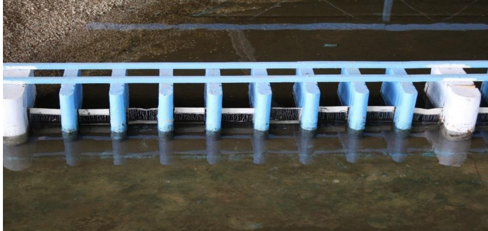
Photo 1: The Trash Rack Simulates 0% Blockage By Aquatic Weeds
