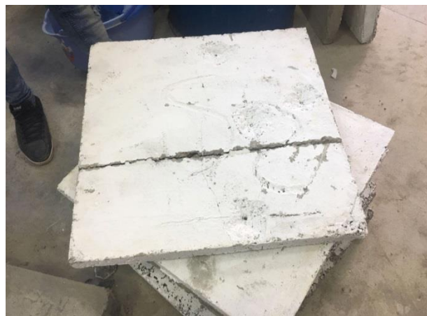
Fig. 25: Slab (S8)with additional 6 Carbon Fiber sheest1*150 mm in both Directions (Fcu =22 mpa Pu=56kn)
