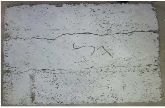
Fig. 18: Reference Slab (S7) with Reinforcement 4Ø6 mm in both Directions (Fcu =22 mpa Pu=12.2kn)
