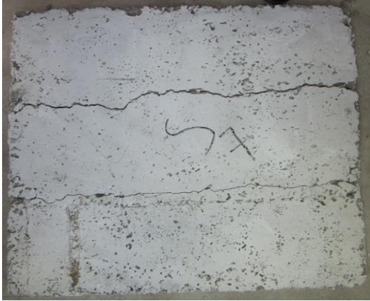
Fig. 18: Reference Slab (S7) with Reinforcement 4Ø6 mm in both Directions (Fcu =22 mpa Pu=12.2kn)
