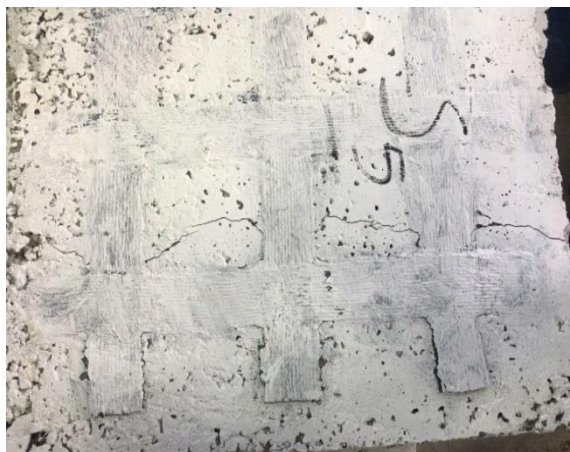
Fig. 24: Slab (S5) with additional 3 Carbon Fiber sheest 1*150 mm in both Directions (Fcu =22 mpa Pu=44.3kn)
