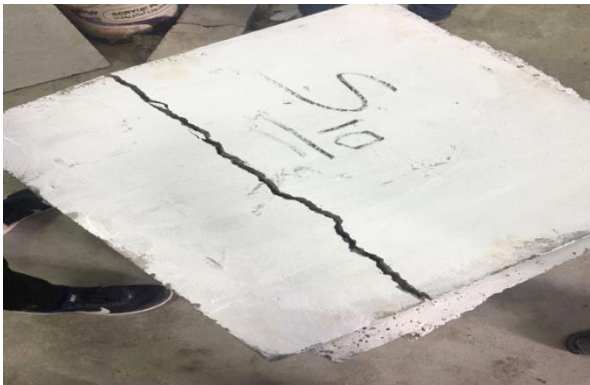
Fig. 22: Slab(S10) with additional reinforcement 6Ø 6 mm in both Directions (Fcu =22 mpa Pu=30.52kn)
