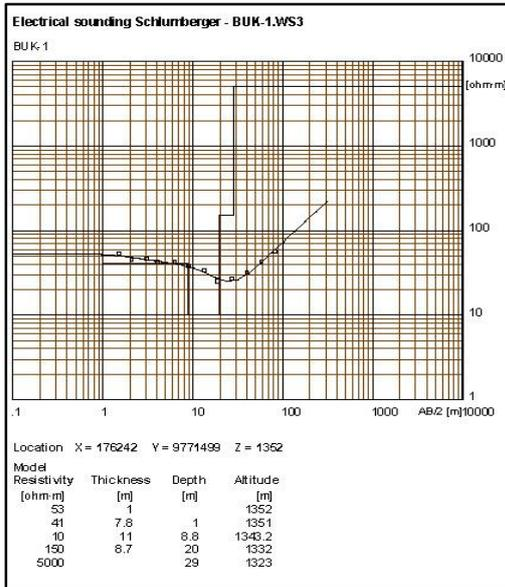
FIGURE 11 ELECTRICAL SOUNDING SCHLUMBERGER- BUK-1
