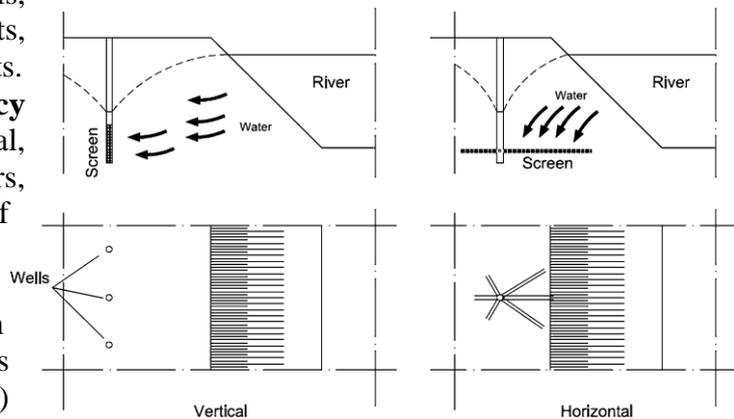
FIGURE 1 HORIZONTAL AND VERTICAL WELLS IN BF SYSTEMS
