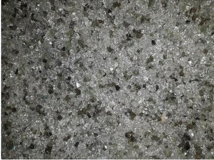
Figure 1. Coarse Glass Aggregates Sample.
