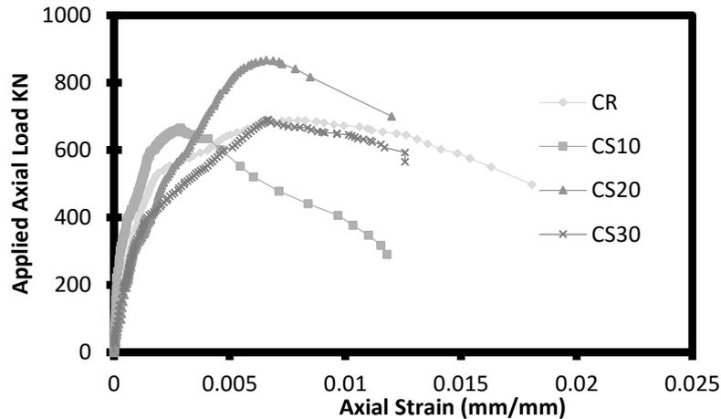
Figure 6b. Axial Strain against Applied Load for control column and columns with fine glass aggregates.
