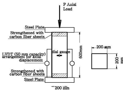
Figure 3. Setup and Concrete Dimensions
