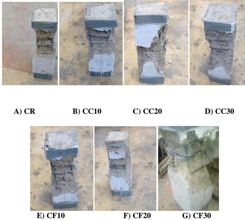
**Figure 5. Crack propagation and failure modes of columns**
