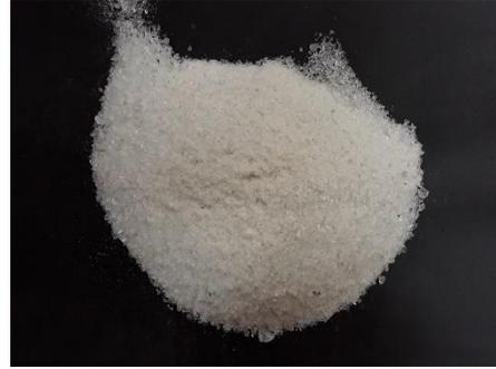
Figure 2. Fine Glass Aggregates Sample
