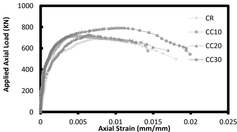
**Figure 6a. Axial Strain against Applied Load for control column and columns with coarse glass aggregates**
