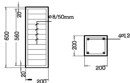
Figure 4. Reinforcement Details of Columns
