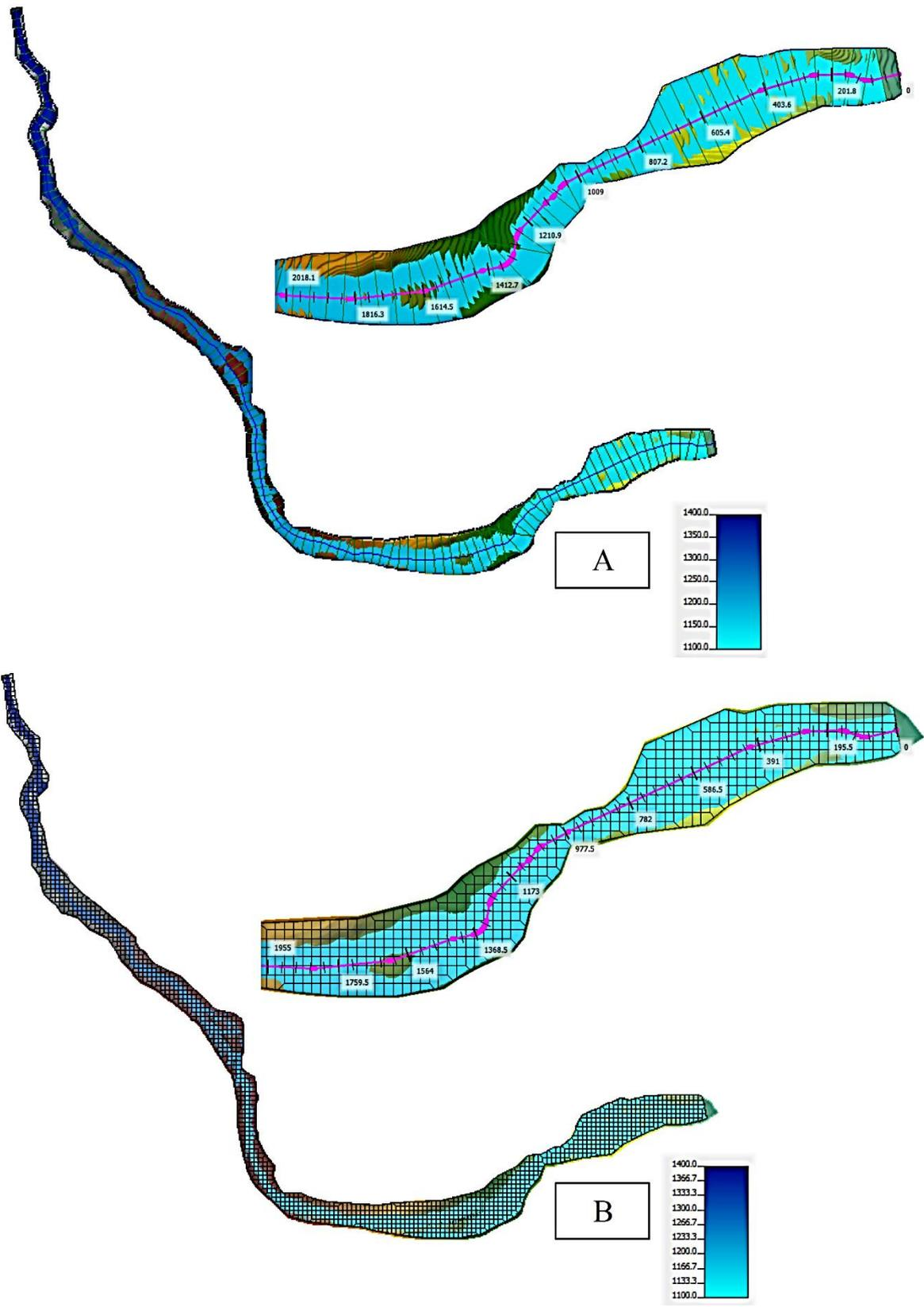
Figure (6) A Comparison of Inundation Map (A) 1D Model (B) Semi 2D Model
