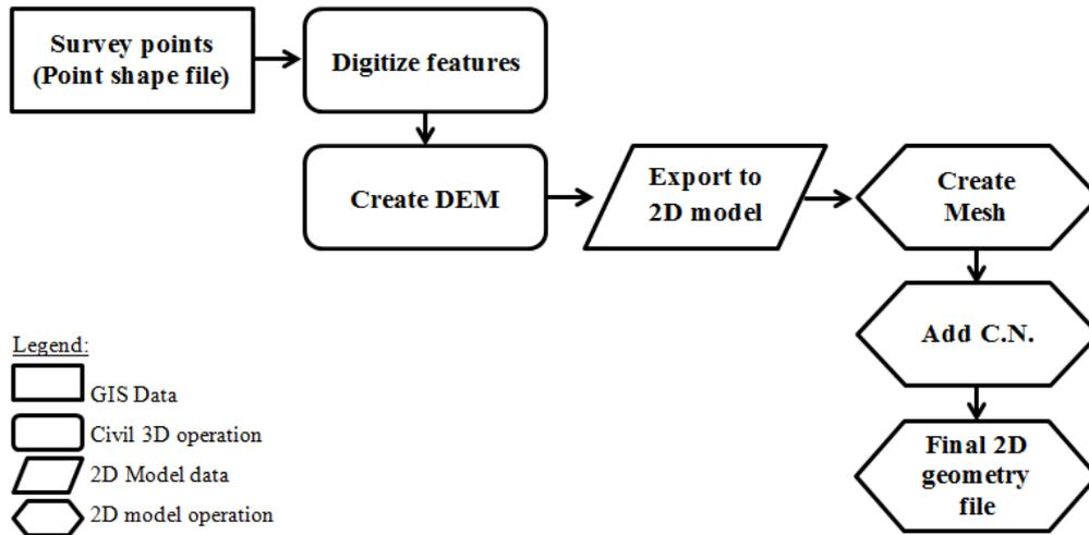
**Figure (4) Work Flow for Developing the 2D and Semi 2D Geometry File**
