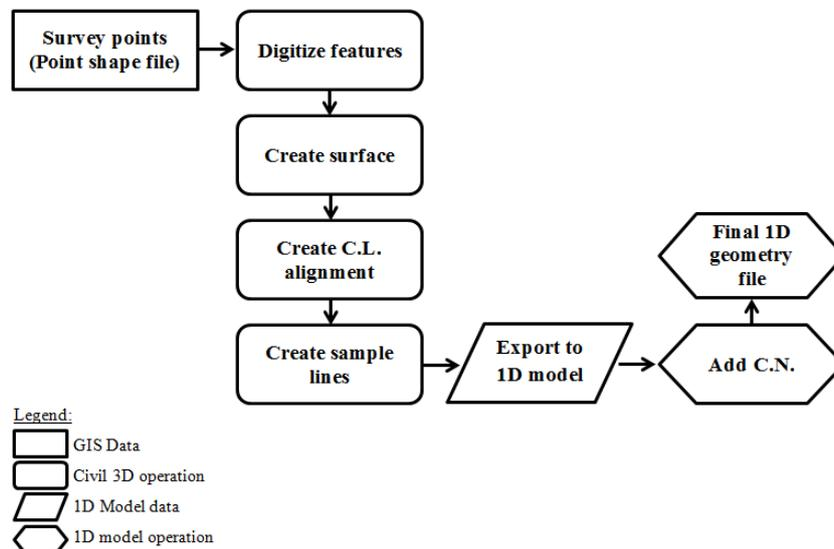
Figure (3) Work Flow for Developing the 1D Geometry File
