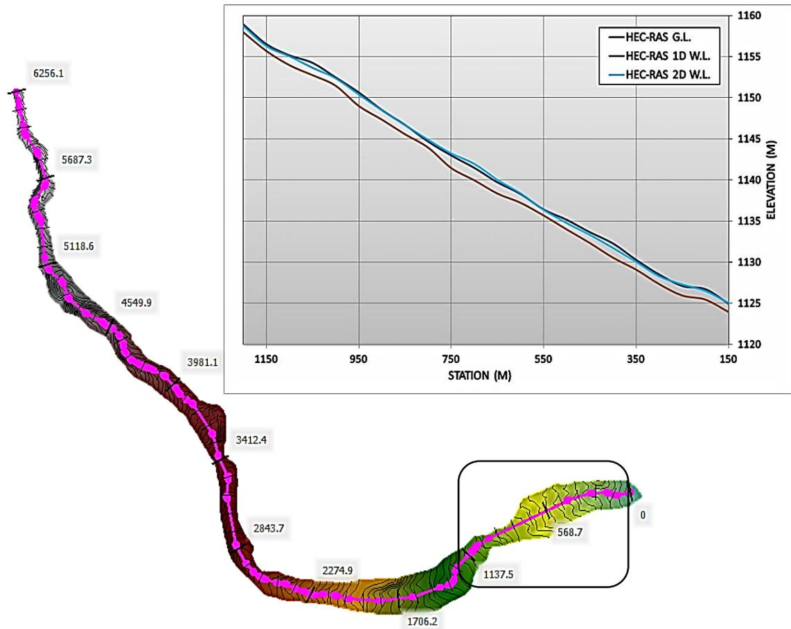
**Figure (5) Maximum WSEL Profile Computed with 1D and Semi 2D Model**
