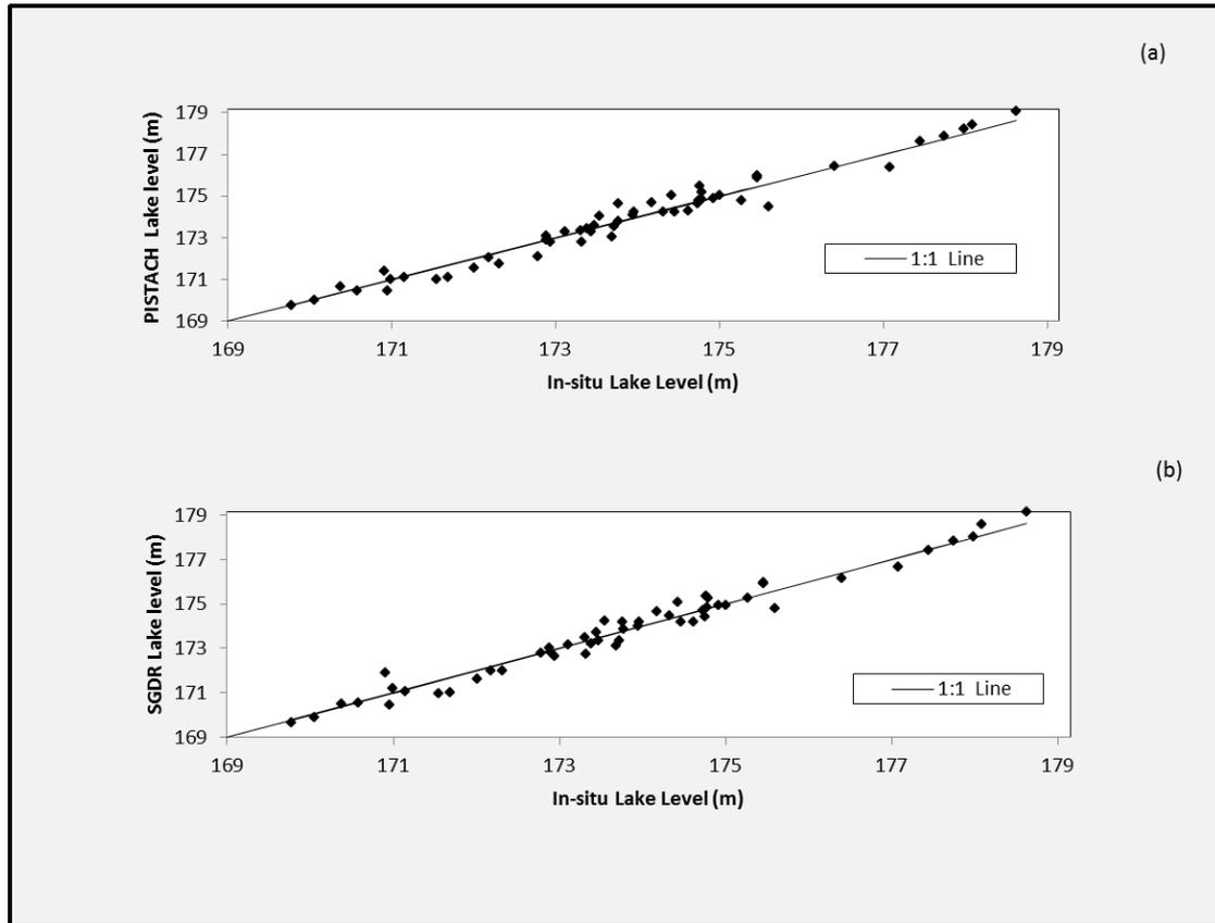
Figure 7. Comparison between monthly mean in-situ measurements and water levels derived using (a) PISTACH and (b) SGDR satellite altimetry datasets
