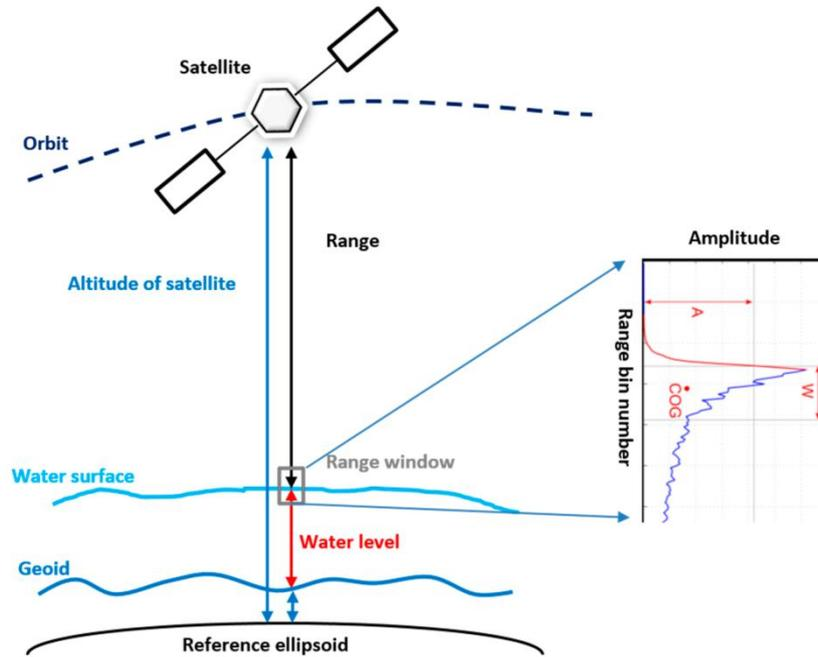
Figure. 1. Altimetry Principle of Water Level Measurement (photo credit[4])
