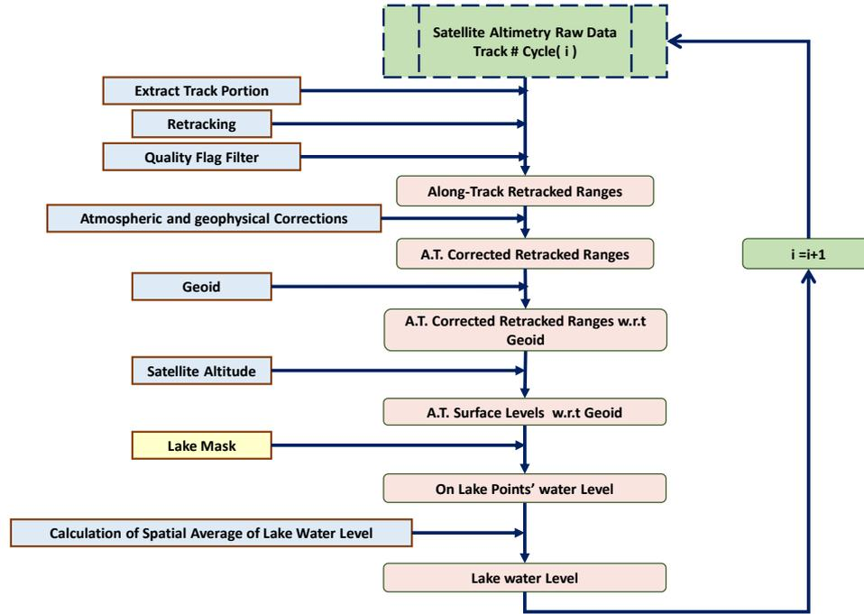
**Figure 2. Schematic of Methodology**
