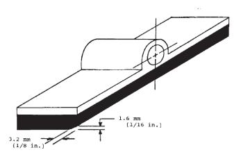
Fig. 3 Slider Assembly Illustrating the Maximum Wear on Striking Edge
