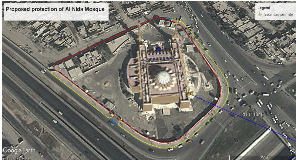
Fig. 7: Proposed barriers around the building [21]
