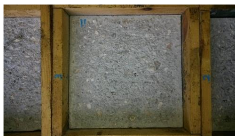
Figure (3): Interface surface profile of hammered test specimen
