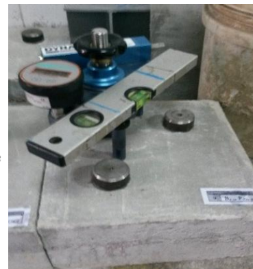
Figure (8): Water bubble levelling of the device base
