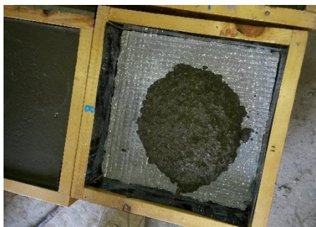
Figure (5): Placing of overlay concrete
