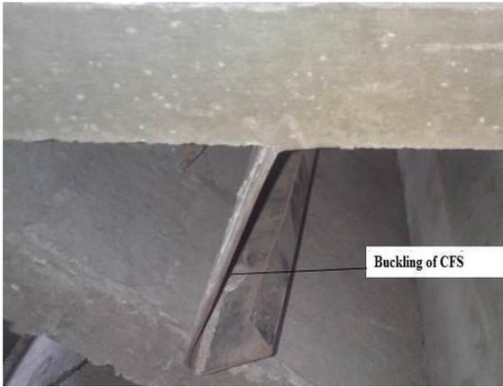
**Figure (11):** Typical large-scale test specimen (b1) failed due to buckling of CFS at support.
