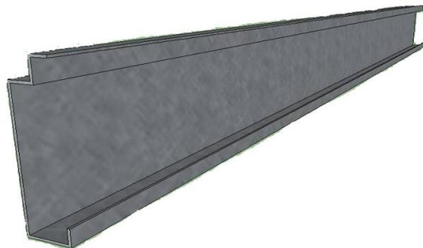
**Figure (1a):** Bent-up half flange of channel along beam as shear dowel.
