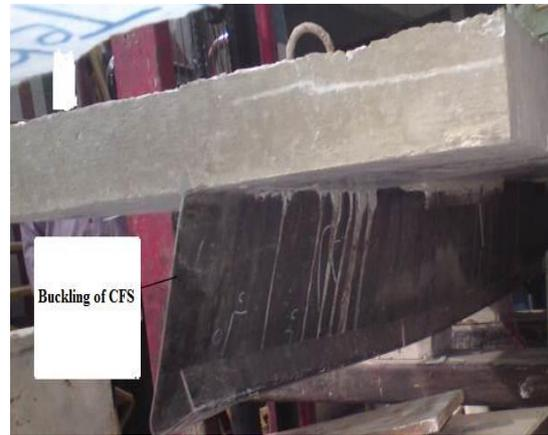
**Figure (14):** Typical large-scale test specimen (b6) failed due to buckling of CFS at support.
