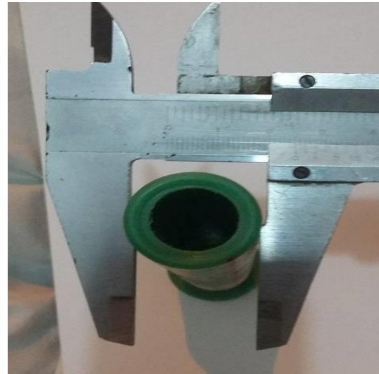
Photo (2): Outer diameter of well
