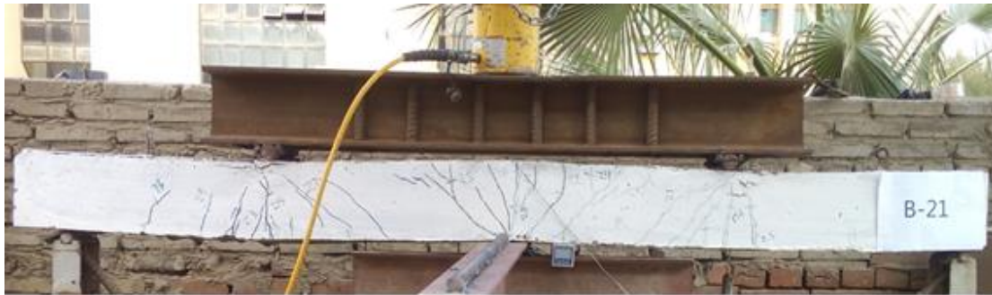
Fig.5 Mode of failure for group 2.
