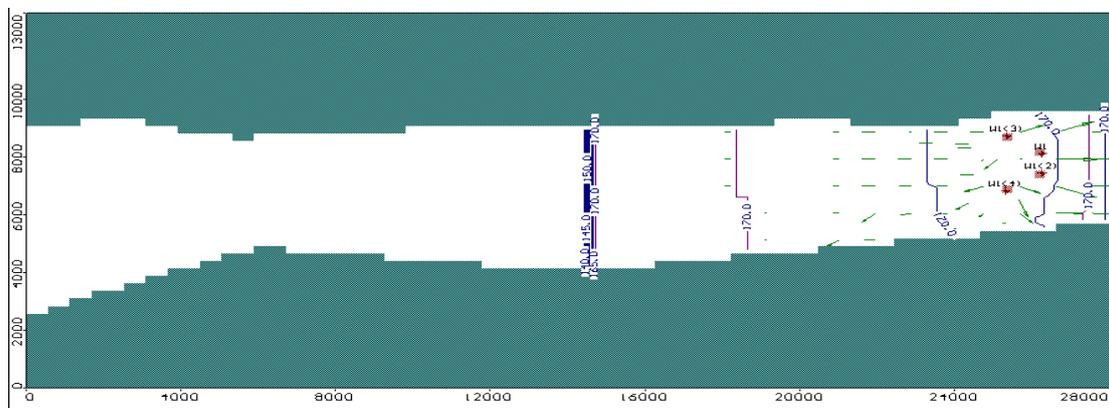
Figure (16): Equipotential lines and velocity vectors in case of using slurry wall
