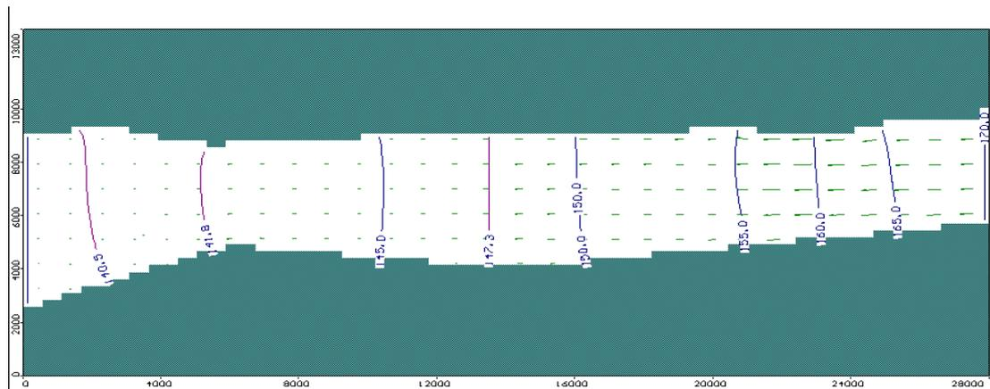
Figure (11): A plan showing Equipotential lines and velocity vectors with the injection and recharge
