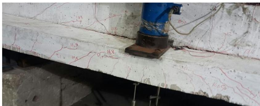
(a) Cracking pattern of the hanger steel failure
