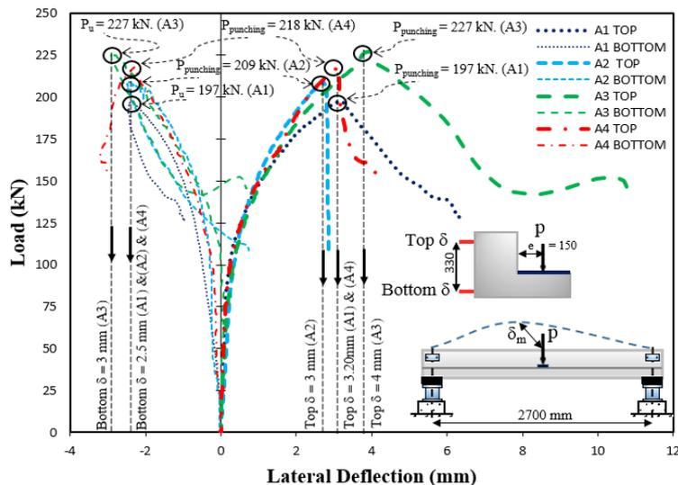
**Figure (14):** Load versus mid-span lateral deflection of beams A1 to A4
