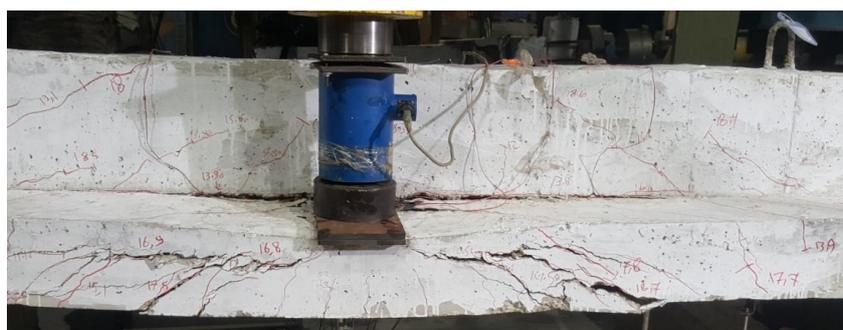
(b) Propagation of the cracks on front of the ledge
