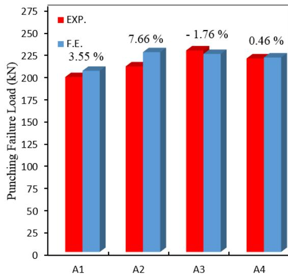
**Figure (20):** Experimental versus F.E. in terms of punching failure loads.
