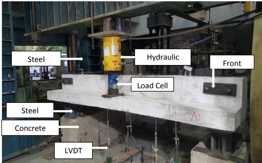
**Figure (6):** Test setup
