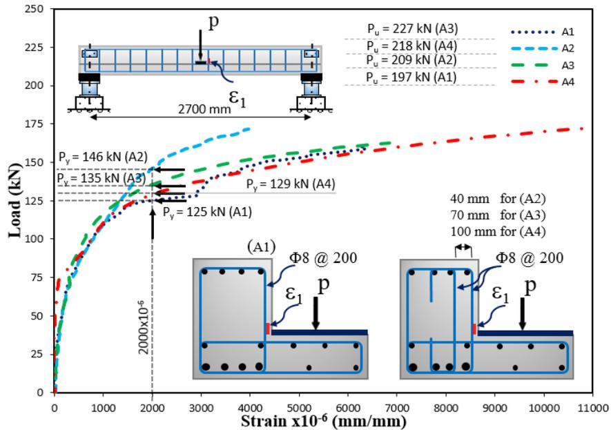
Figure (15): Load versus strains of outer stirrups ( $\square_{\square}$ ) at mid-span of beams A1 to A4
