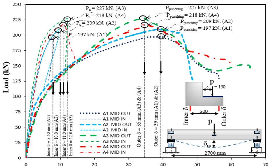
**Figure (12):** Load versus mid-span vertical deflection of beams A1 to A4
