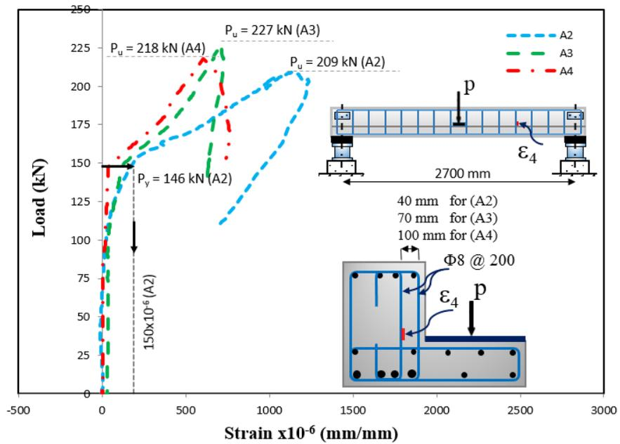
**Figure (18):** Load versus strains of inner stirrups ( $\square$ ) at quad-span of beams A1 to A4
