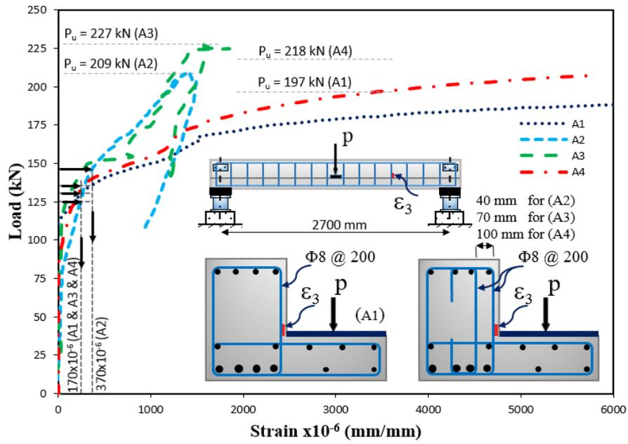
**Figure (17):** Load versus strains of outer stirrups ( $\square$ ) at quad-span of beams A1 to A4
