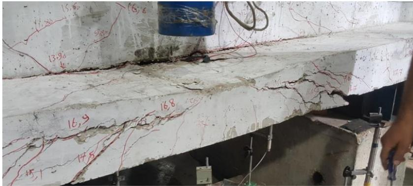
(c) Cracking pattern of punching failure
