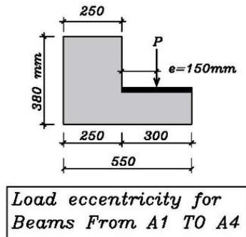
**Figure (7):** Load eccentricity for specimens
