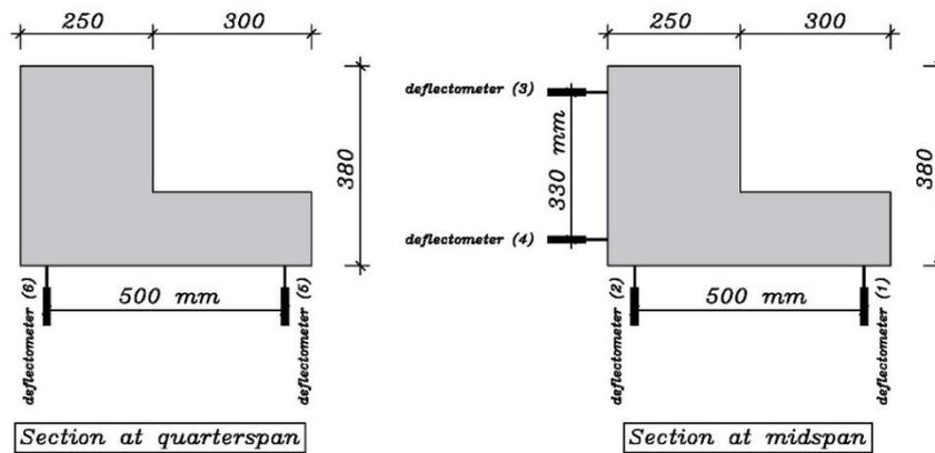
**Figure (9):** Location s of deflectometers for tested beams
