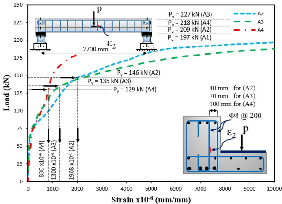
Figure (16): Load versus strains of inner stirrups ( $\square_{\square}$ ) at mid-span of beams A1 to A4
