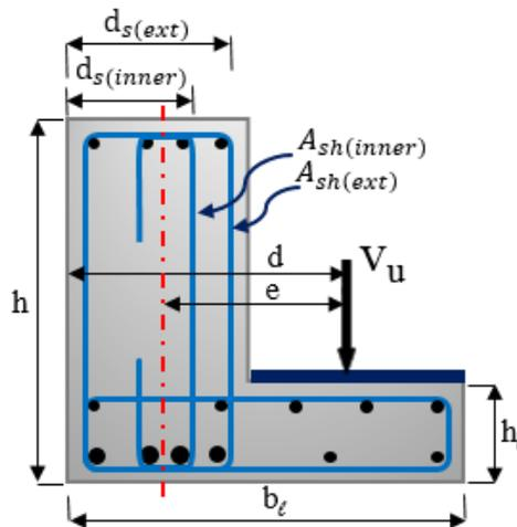
**Figure (10):** Design of hanger steel reinforcement
