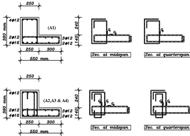
**Figure (8):** Locations of steel strain gauges for tested beams
