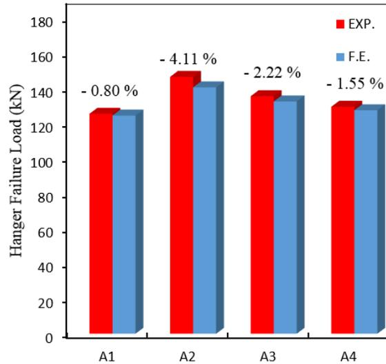
**Figure (19):** Experimental versus F.E. in terms of hanger failure loads.
