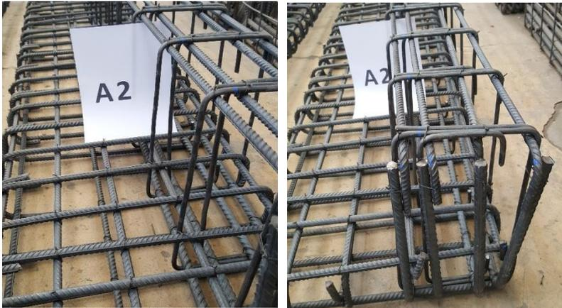
Figure (2): Concrete Dimensions and Reinforcement Details for Beam (A2)
