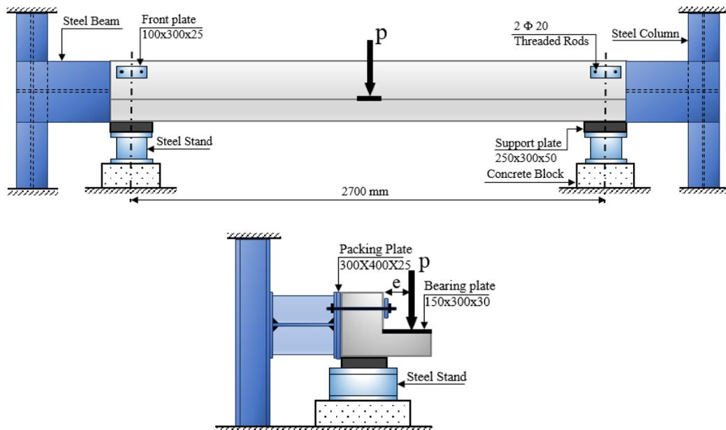
**Figure (5):** Loading setup for tested beams
