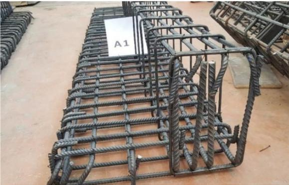
Figure (1): Concrete Dimensions and Reinforcement Details for Beam (A1)
