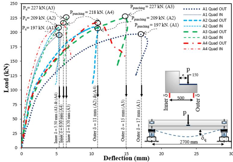
**Figure (13):** Load versus quad-span vertical deflection of beams A1 to A4
