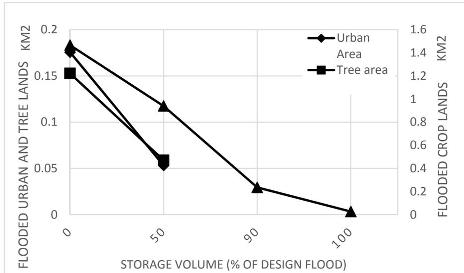
**Figure 8 Reduction in affected areas due to storing flood water partially in the upstream of the study area.**
