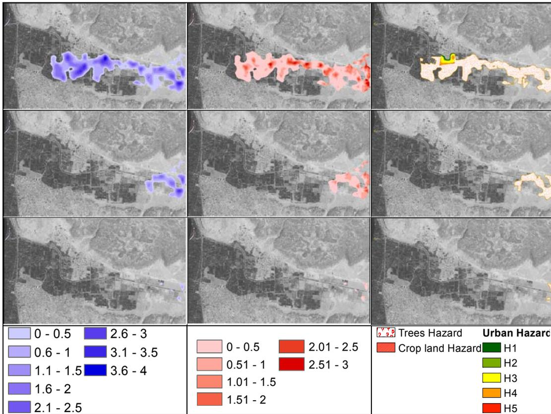
Figure 7 the coloured areas represent the spatial distribution of maximum depth (left column), the spatial distribution of maximum velocity (middle column), and the spatial and degree distribution of flood risks over different land uses in the study area.
