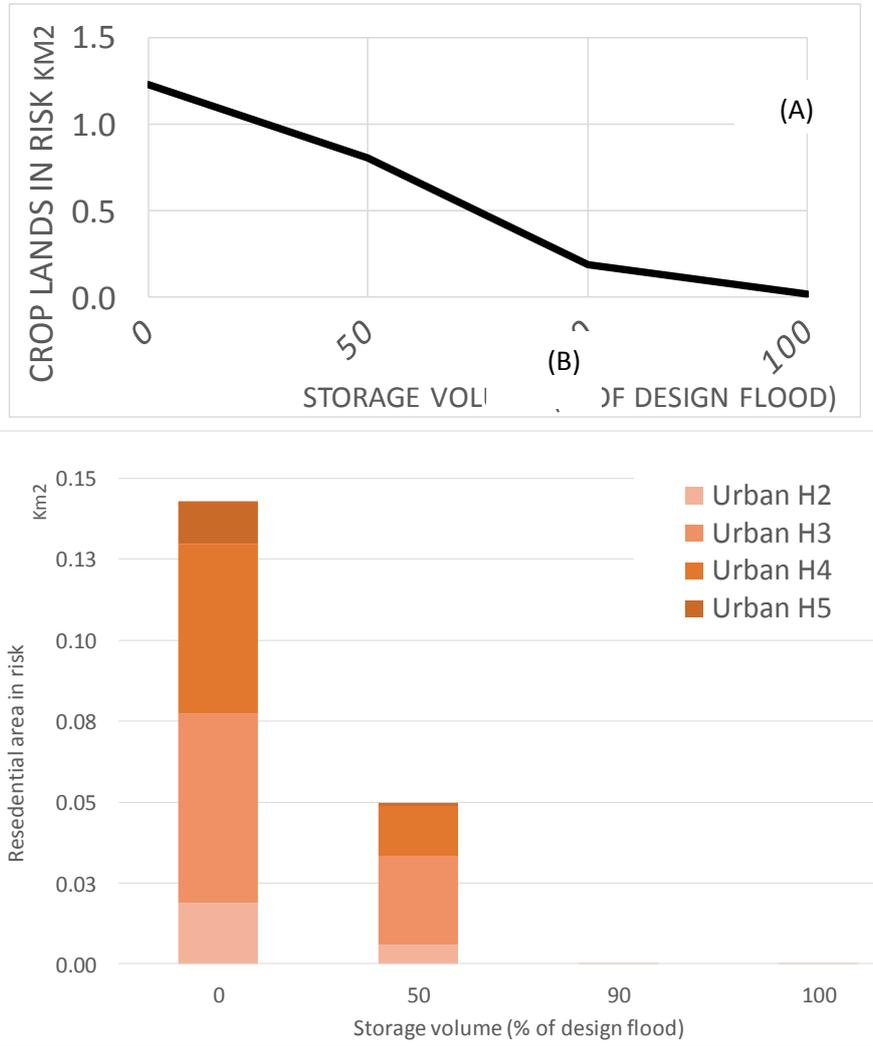
Figure 9 Crop areas under risk w.r.t. each proposed flood protection structure (left), noticing that Urban H1 and Urban H6 were ignored because the first one doesn't cause any harm
