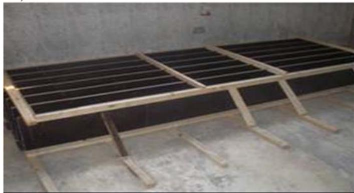
**Figure 6:** Formwork of the tested beams
